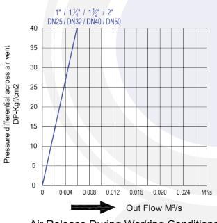
Air Release During Working Conditions Small orifice
