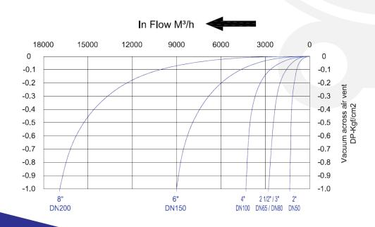
Gamma HPTM automatic air flowing out capacity, at high pressure, by size:
